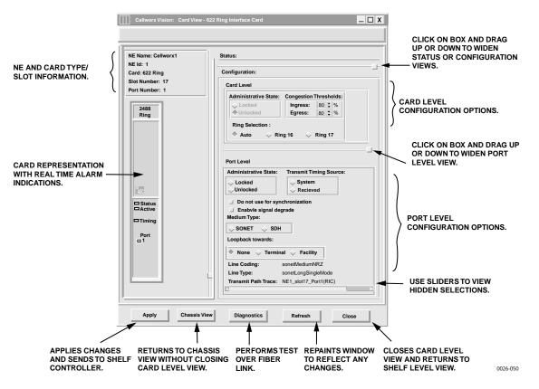
Figure 756-1. 2488 RIC Shelf Level GUI Configuration Screen
